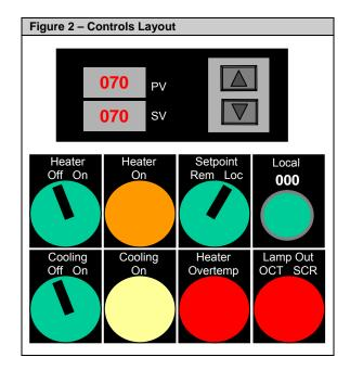
The control box contains a PLC control, which allows "smart" alarming. Table 1 displays the function of the indicator lights.
