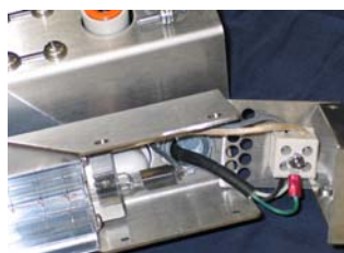
↑↑ Water Cooled Line & Strip heaters using short-wave ↑↑ IR emitters. Utilizes a highly polished custom aluminum extrusion, easy access covers for wiring and lamp access, quick-push-connect water fittings, easy mount t-slots and optional quartz window and multi-axis mounting brackets. Available in 5, 10, 16, 25, 38" lighted lengths.
