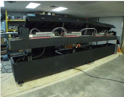
← 6 Meter long, Adjustable Height, 4 Zone IR Oven & Controls. Uses PCS designed water-cooled strip heaters, Allen-Bradley PLC and Operator Interface. ←
