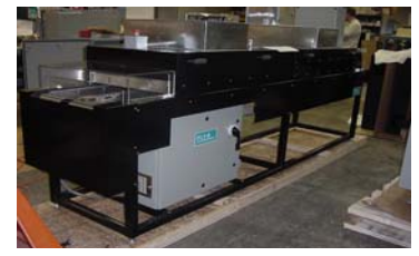
↑↑ 120" long, 28" wide, multi-zone heating, conveyorized drying oven & controls. Adjustable speed & temperature settings with pyrometer feedback
