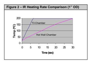
In the example, the faster heating capability of the T3 lamp system provides benefits of either:
